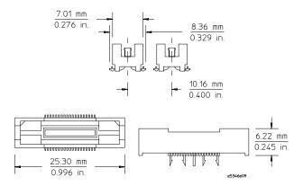
38-pin MICTOR connector dimensions
