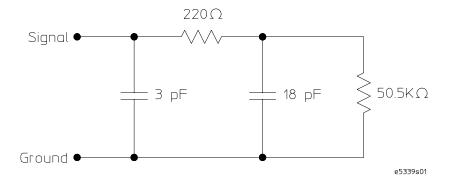
Equivalent probe load
